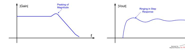
45° pole-pair angle corresponds to  $Q = \frac{1}{\sqrt{2}}$ 90° pole angle (on pole pair) corresponds to  $Q = \frac{1}{2}$
