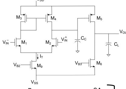
$$\begin{array}{lll} 4\beta \ A_0 > \frac{p_2}{p_1} > 2\beta \ A_0 & \Longrightarrow k & \cong \frac{\beta A_{0TOT}}{Q^2} \\ p_2 = \frac{g_{00}}{C_L} & p_1 = \frac{g_{0d}}{C_C} & A_0 = \frac{g_{m0}g_{md}}{g_{00}g_{0d}} \end{array}$$
