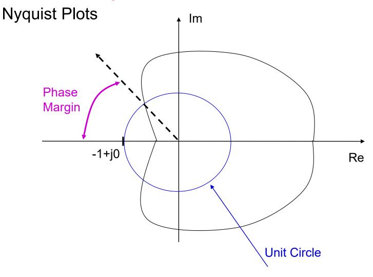
Phase margin is  $180^{\circ}$  – angle of A $\beta$  when the magnitude of A $\beta$  =1
