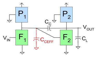
$$A(s) = \frac{g_{md}(g_{m0} - sC_C)}{s^2 C_C C_L + sg_{m0} C_C + g_{oo} g_{od}}$$
